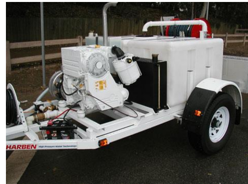
Harben Hydro-jet Trailer
