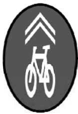
Recommended Shared Lane Marking 11' (min) center to curb
