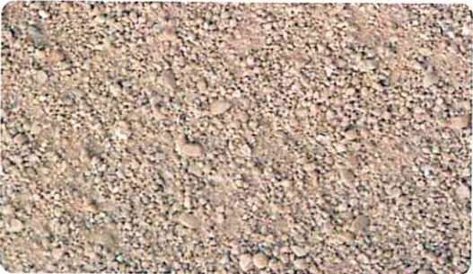
DECOMPOSED GRANITE (DG) STABILIZED
