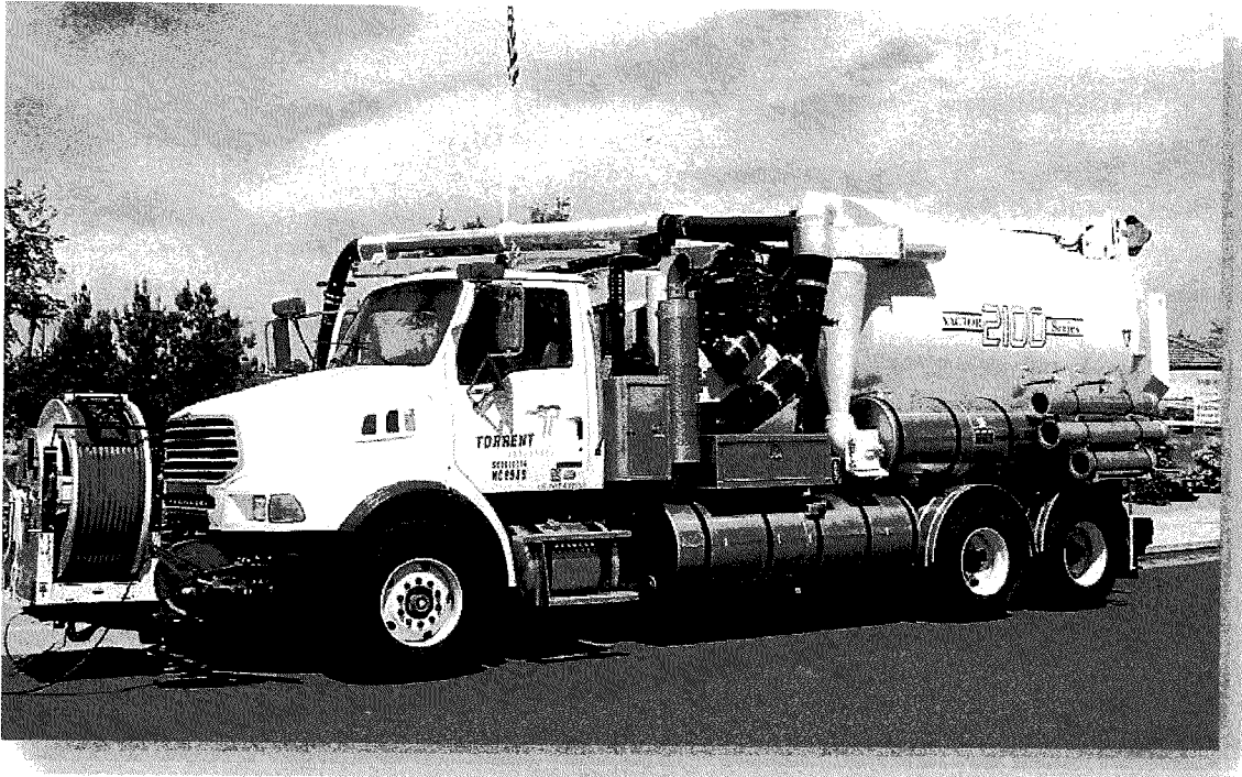
Typical hydro-vacuum truck used for drywell maintenance
