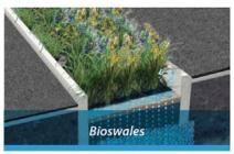
New parkway bioswales in the median Natural materials will be utilized in with native planting materials, grasses, flowers, trees and shrubs provide vegetated areas through which stormwater will be filtered, resulting in the removal of pollutants and groundwater replenishment.
