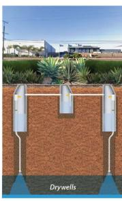
Drywells are an infiltration best management practice (BMP) designed to capture, treat and infiltrate stormwater runoff. They can also provide flood mitigation.
