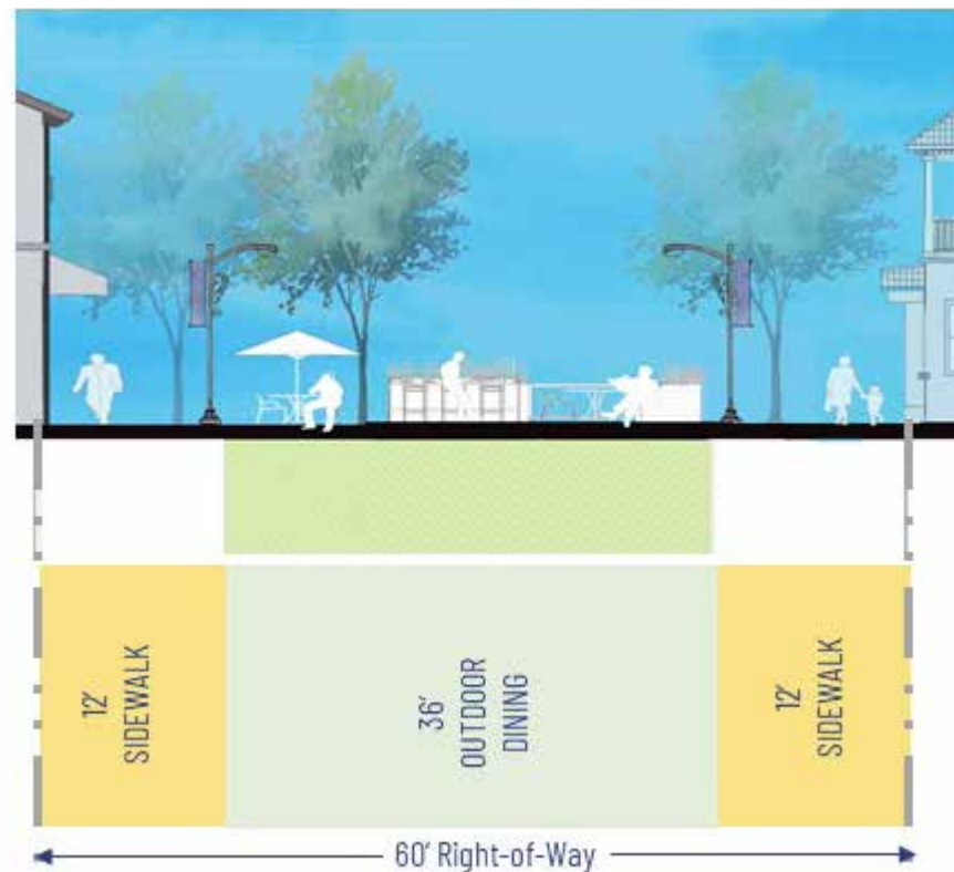
Figure 3.15 Richmond Street Alternative Road Section
