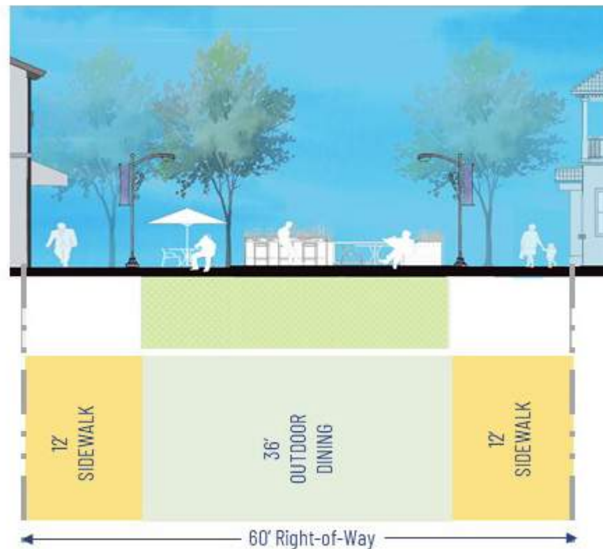
Figure 3.15 Richmond Street Alternative Road Section
